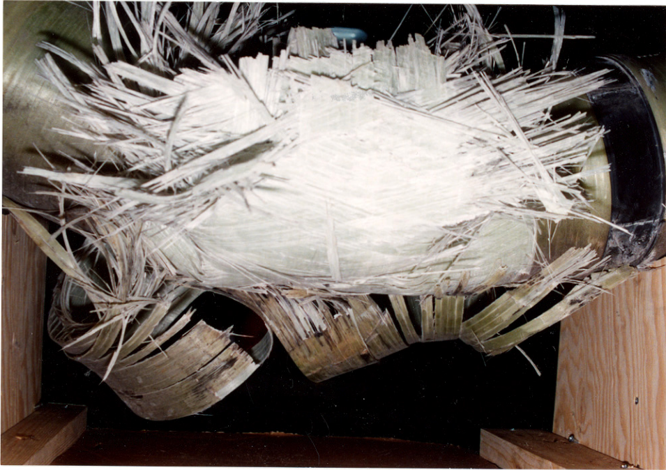
47. View of the top left surface of the fractured composite wrap looking toward the forward end of the tank along the right side of the photograph
